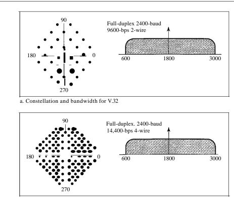
Figure 9.8 The V.32 and V.32bis constellation and bandwidth
