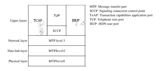
Physical Layer: MTP Level 1 The physical layer in SS7 called message transport part (MTP) level I uses several physical layer specifications such as T-l (1.544 Mbps) and DCa (64 kbps).
