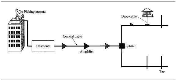
The cable TV office, called the head end, receives video signals from broadcasting stations and feeds the signals into coaxial cables. The signals became weaker and weaker with distance, so amplifiers were installed through the network to renew the signals. There could be up to 35 amplifiers between the head end and the subscriber premises. At the other end, splitters split the cable, and taps and drop cables make the connections to the subscriber premises.
