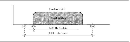
The term modem is a composite word that refers to the two functional entities that make up the device: a signal modulator and a signal demodulator. A modulator creates a bandpass analog signal from binary data. A demodulator recovers the binary data from the modulated signal.
